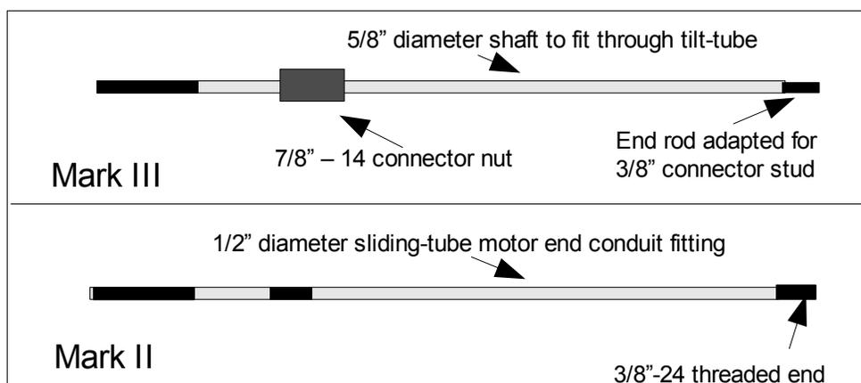
To replace the cable, remove the pump cover as explained in shift cable replacement. Disconnect cable end fitting and remove billows. If it is a MARK III, unscrew the cable housing nut, then the adapter nut. Twist the adapter to break the seal and remove from the cable. If it is a MARK II, unscrew the adaptor nut and twist the adaptor CCW to loosen. Continue to twist as the adaptor is threaded to the cable housing.
